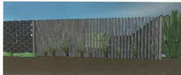
VERTICAL LOUVERED STEEL WALL
