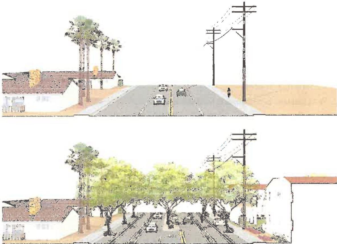
Example of a complete street transformation along Avenue 44 (existing street above, complete street below).
