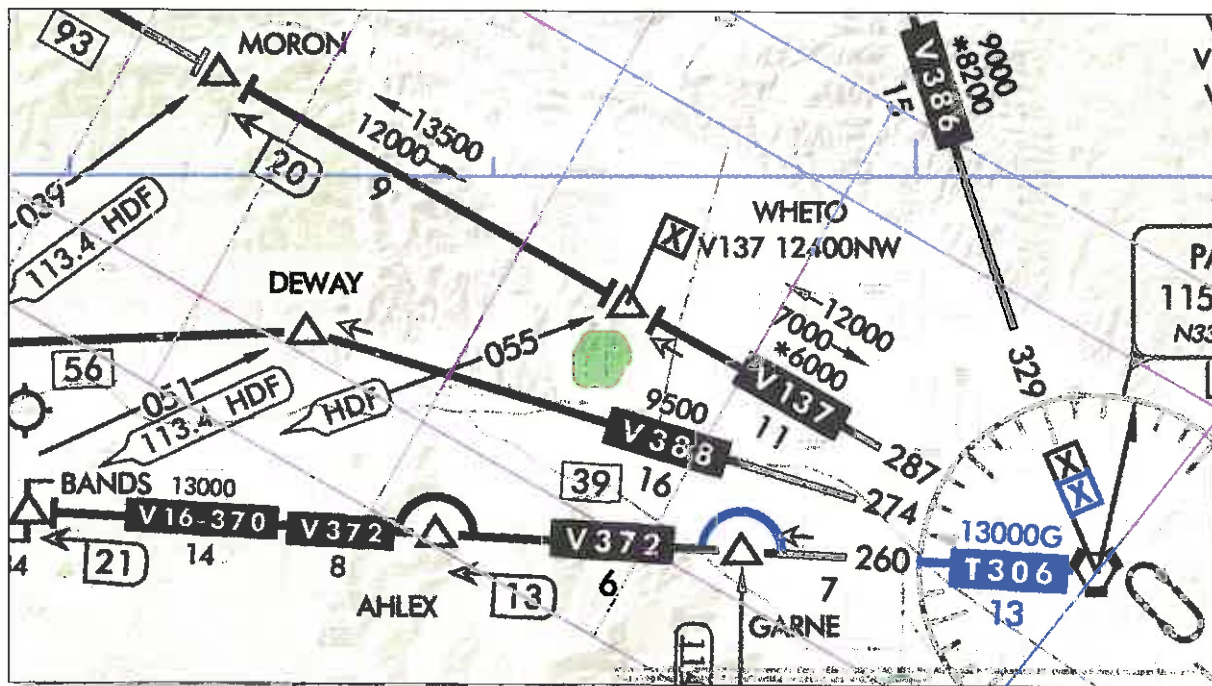
Figure 6: Low altitude enroute chart L-4 with V137 obstacle evaluation area (purple)
