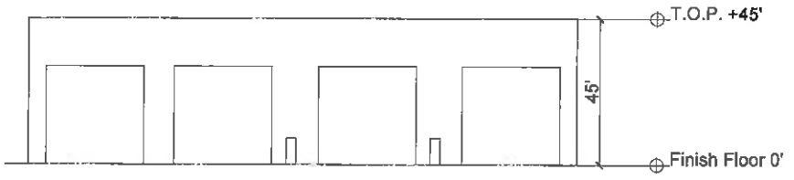
3 NEW HANGAR BUILDING - ELEVATION 3 1/16" = 1'-0"
